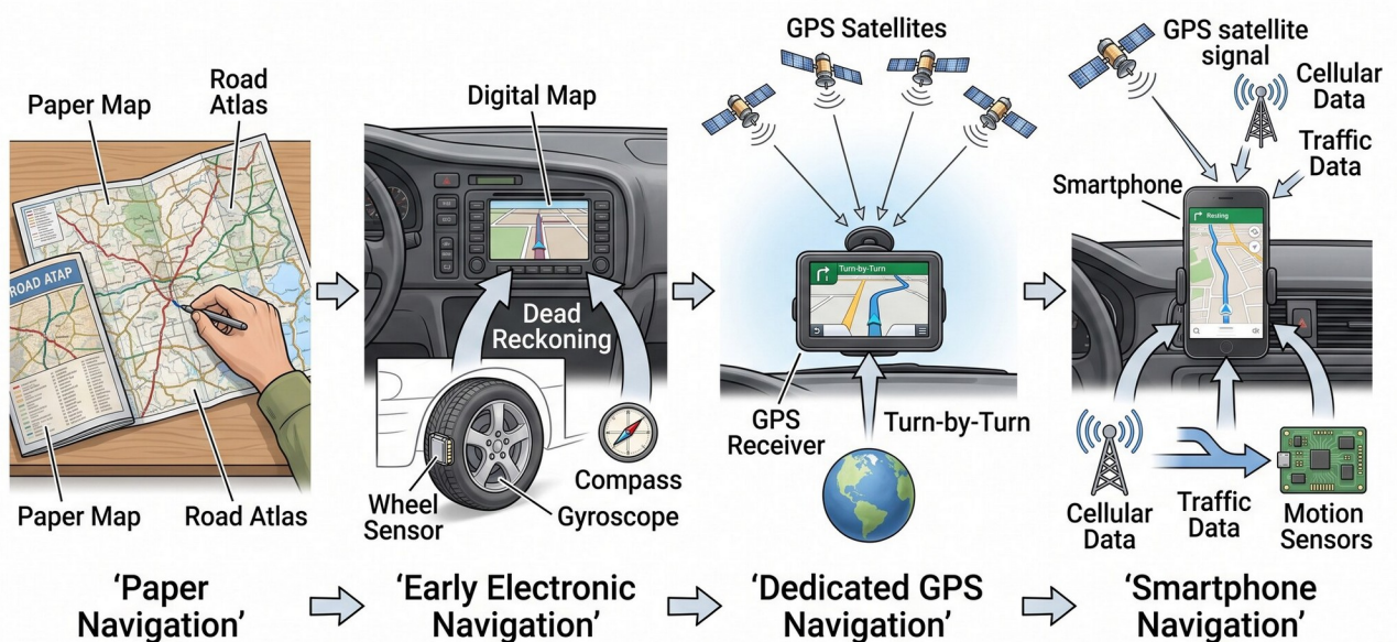
Figure 3. Electronic navigation evolved by combining digital maps with increasingly accurate ways of estimating or measuring vehicle position.
